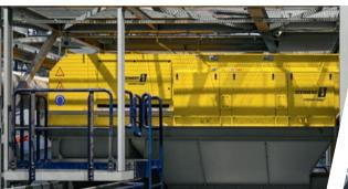
Removal of ferrous metals using STEINERT UME
